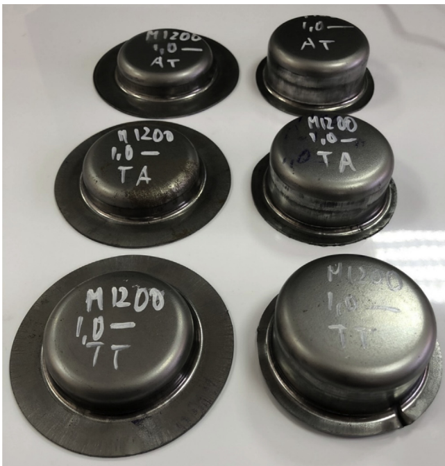
Fig. 13. Manufactured parts: M1200; 1.0 mm thickness; blank-holders TS, ST and TT.
