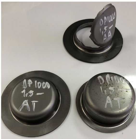
Fig. 10. Manufactured parts: DP1000; 1.5 mm thickness; blank-holders ST and SS (failure in first step).
