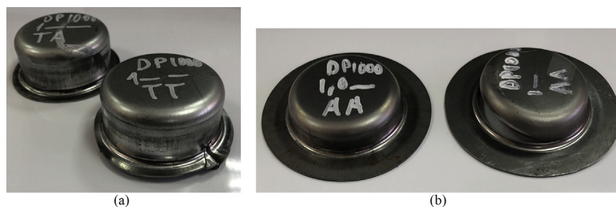
Fig. 7. Manufactured parts. (a) DP1000; 1.0 mm thickness; blank-holders TS and TT; (b) First step and second step (failure) with blank-holders SS.
