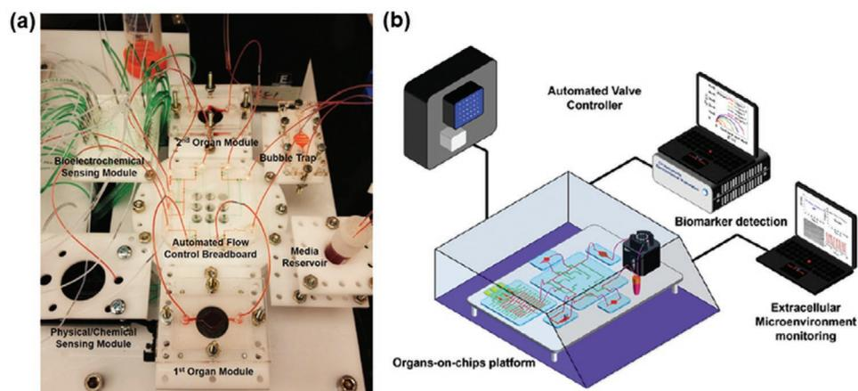
**Figure 8.** Multisensor-integrated organ-on-a-chip platforms for automated and continuous in situ monitoring of organoids. a) Photograph of the integrated platform including microbioreactors, breadboard, reservoir, bubble trap, physical sensor and electrochemical biosensors; b) Schematic of the full system organ-on-a-chip platform enclosed in an in-house designed benchtop incubator. Reproduced with permission.<sup>[132]</sup> Copyright 2017, PNAS.
