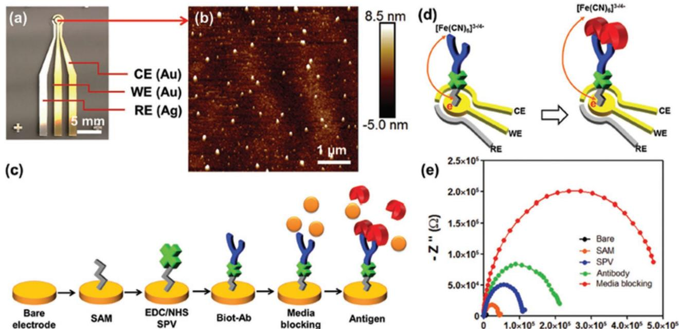
**Figure 9.** Label-free EC biosensing system for continuous measurement of cell-secreted biomarkers from an organoid cultured of a human liver-on-a-chip. a) Photograph of the microelectrode; b) AFM image of the bare working electrode surface; c) schematic illustration of the antibody immobilization on the surface of the microelectrodes; d) Nyquist plots after antigen binding upon antibody-antigen. Reproduced with permission.<sup>[23]</sup> Copyright 2017, Wiley-VCH.
