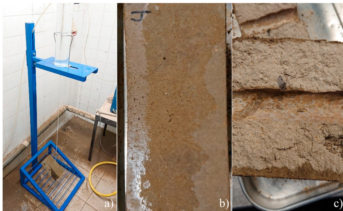
Fig. 9. Swinburn test setup (a); surface of the CEB after exposure (b); water penetration depth (c).
